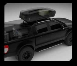
A covert surveillance 4x4 pickup vehicle is equipped with the AARTOS<sup>™</sup> System and a concealed IsoLOG<sup>®</sup> 3D RF Antenna Array. This setup includes optional jamming capabilities and features a single operator station located on the back seat, designed for stealth and efficiency.
