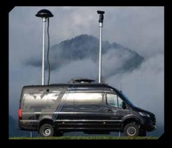
The AARTOS<sup>™</sup> Drone Detection System is seamlessly integrated into a 4x4 Mercedes Sprinter, equipped with enhanced features such as an optical and thermal PTZ camera, a satellite uplink and a northfinder antenna. This setup includes a dual operator compartment with four 4K monitors and highend hardware, providing a comprehensive surveillance and operation platform.
