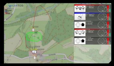
A top-down 2D perspective is the most commonly used visualization technique in drone detection. The 3D view expands our capabilities by adding the drone's altitude information.
