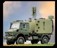
An all-terrain vehicle solution, self-sustaining and equipped with the AARTOS<sup>™</sup> shelter integration, features the lsoLOG<sup>®</sup> 3D RF antenna array and an optional upgrade for a 40 km long-range antenna.
