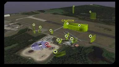
Using an (optional) sophisticated radar system, the AARTOS™ DDS can automatically determine and display the exact position, flight direction, altitude, speed and classification of an inbound drone.
