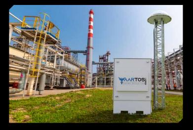
AARTOS<sup>™</sup> Stationary Drone Detection installations, which can incorporate either the AARTOS<sup>™</sup> X7 or X9 models, are adept at establishing freely scalable detection grids. These systems are designed for extensive coverage: for instance, three X7 units can cover approximately 220 square kilometers, while three standard X9 units extend the coverage to over 1700 square kilometers. Key features of these installations include remote controllability and fully auto-
