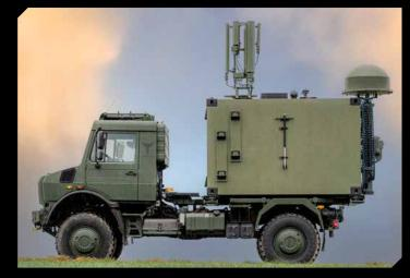
The Zeppelin FM1 and he Zeppelin FM2, these shelters are manageable and can be transported via Unimog or similar vehicles. Versatile for both mobile and stationary use, manned or remote operation, the AARTOS<sup>™</sup> Drone Detection shelter serves as an effective solution for professional airspace monitoring to identify and intercept unauthorized drones.
